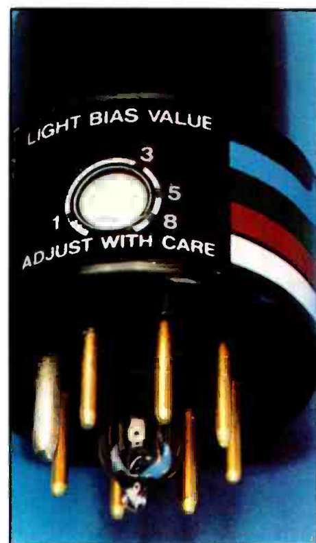
Bias lighting to reduce lag may be adjusted through an in-base control on some tubes.
